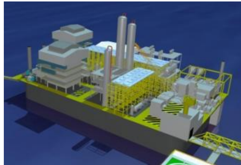
Methanol Plant on GBS
